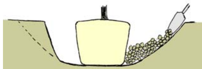
Figure 3. A labor-saving technique is to widen the planting hole into the desired saucer shape, three times the root ball diameter during the during backfill process.
